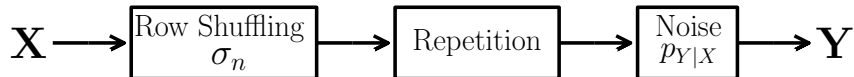
Fig. 2. Relation between the unlabeled database \mathbf{X} and the correlated repeated database \mathbf{Y} . Repetition is represented by the repetition pattern S^n (Definition 2) or the repetition matrix \mathbf{S} (Definition 3).
